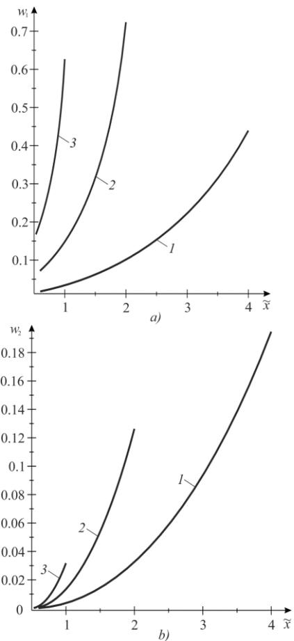
Fig. 5. Graphical dependencies of length of plastic strip at the crack tips on relative coordinate of crack centre  $\tilde{x}_0 = x_0/l$  at various values of external load
