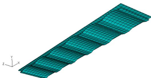
Fig. 8. FEM model of the assembly of foils
