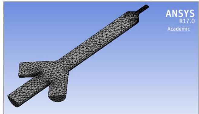
Fig. 6. Finite element mesh of extrusion nozzle flow channels
