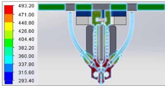
Fig. 3. Results of thermal analysis without external cooling
